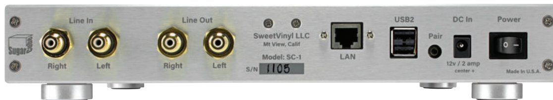
The rear panel carries chunky gold plated RCA phono socket inputs and outputs (at left), an RJ45 ethernet LAN socket, USB sockets and a 12V d.c. input for connection to the external power supply. Note also the crucial Pair button used during set up, situated between USB and d.c. sockets.
